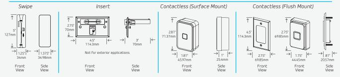
Swipe Reader: Insert Reader: Contactless Reader (Surface Mount): Contactless Reader
