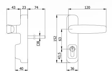
CONSTRUCTIVE FEATURES: Painted special alloy case and handle -Zinc and plastic plated steel cover - Nickel-plated brass cylinder. WORKING: Door opened by the handle - Handle interlock is controlled by the key (free handle).
