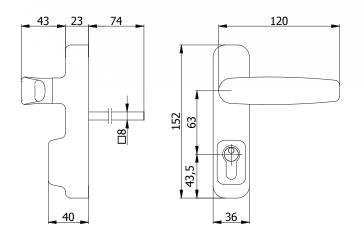
CONSTRUCTIVE FEATURES: Painted special alloy case and handle -Zinc and plastic plated steel cover - Nickel-plated brass cylinder. WORKING: Door opened by the handle - Handle interlock is controlled by the key (free handle).
