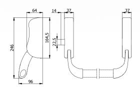
CONSTRUCTIVE FEATURES: Zinc-plated steel cases - Painted aluminium covers - Painted special alloy levers - Chromed special alloy latch bolt - Stainless steel springs.
