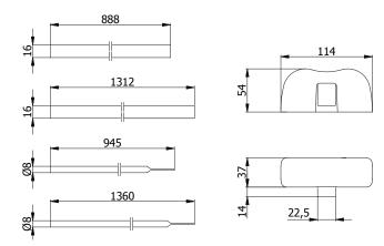
CONSTRUCTIVE FEATURES: Zinc-plated steel cases - Painted aluminium covers - Chromed special alloy latch bolts - Stainless steel springs - Zinc-plated steel rods - Painted aluminium cover rod.
