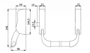
CONSTRUCTIVE FEATURES: Zinc-plated steel cases - Painted aluminium covers - Painted special alloy levers - Chromed special alloy latch bolt - Stainless steel springs.
